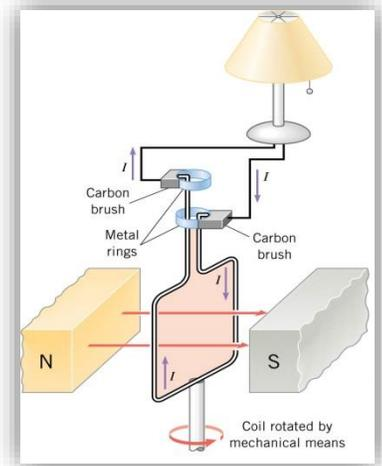
You have made a simple generator to power a TV. The armature is attached the rear axle of a stationary bike. For every time you peddle, the rear axel turns 10 times. Your TV needs a  $V_{rms}$  of 110V to operate. If the  $B$ -field is 0.2 T, each loop is a circle with  $r = 3$  cm, and you can comfortably peddle 3 times a second; how many loops must you have in your generator so that you can watch TV while you exercise?
